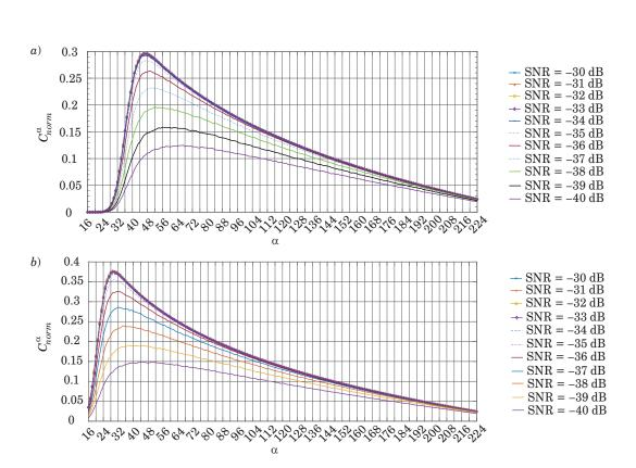
**Fig. 5.** Normalized capacity of the equivalent  $(\alpha, p)$ -channel vs.  $\alpha$  for q = 256, K = 500, various SNR values and Scenario 1 (a) and Scenario 2 (b)
