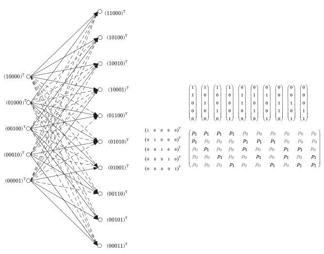
**Fig. 2.** The equivalent  $(\alpha, p)$ -channel diagram and transition matrix (for q = 5 and  $\alpha = 2$ )
