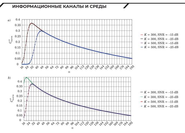
**Fig. 3.** Normalized capacity of the equivalent  $(\alpha, p)$ -channel vs.  $\alpha$  for q = 256, various values of *K* (number of interfering users), SNR and Scenario 1 (*a*) and Scenario 2 (*b*)
