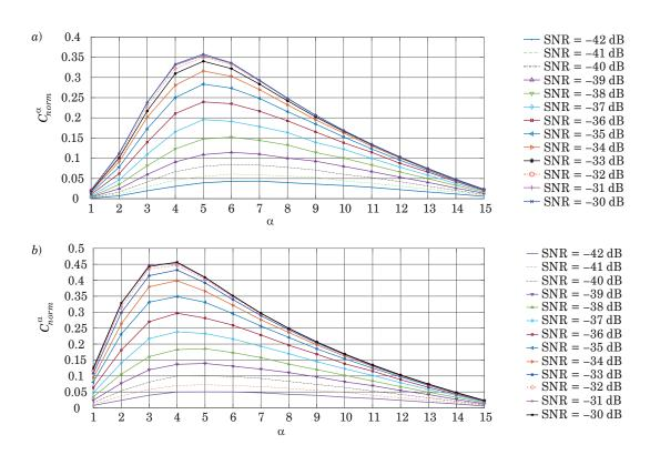
*Fig. 6.* Normalized capacity of the equivalent  $(\alpha, p)$ -channel vs.  $\alpha$  for q = 16, various SNR values and Scenario 1 (a) and Scenario 2 (b)
